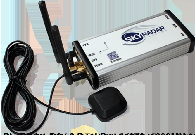
SKYRADAR 1090ES (978-1090MHz) Receiver (based on SkyRadarDX but without AHRS) purchased separately
